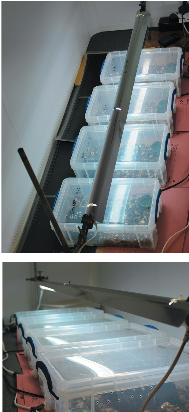
Figure 3. (a) Overhead view, showing lighting positioning over the middle of a row of Really Useful boxes, housing P. muticus . (b) Horizontal view, showing UV-B tube positioned 9 cm above the lids of Really Useful boxes, housing Indian giant scorpions.
